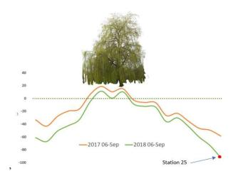
In September 2017, Station 25 was 58.4mm below the datum. 12 months later, the figure was 92.4mm.
